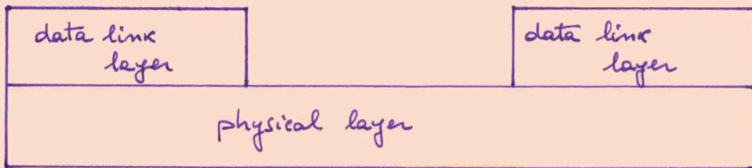
The physical layer is responsible for the transmission and reception of raw data between a device and a physical transmission medium.
